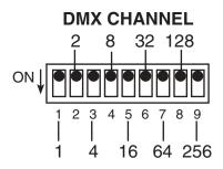
Each dip switch has a preset value, a desired DMX address is set by combining the dip switches that will create your desired value. For example: To achieve a DMX address of 21, combine dip switches 1, 3, and 5. Sense dip switch 1 has a value of 1, dip switch 3 has a value of 4, and dip switch 5 has a value of 16, the combination of the create a DMX value of 21.
